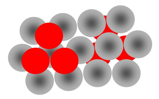
Atoms arrange into close-packed structures due to lack of directional dependence of interaction. Materials with **Metallic** bonding also adopt this structure.
