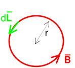
The electric flux through the path is  $\Phi = (Field)(Area) = E_0 sin(\omega t)\pi r^2$
