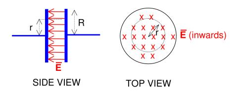
The current flowing across the capacitor, I = 0 (plates are separated by a vacuum or insulator).
