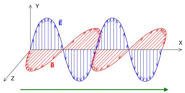
The whole pattern moves in x-direction with speed c
