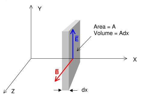
The electromagnetic energy in the slab is:  $dU = \frac{1}{2} \left[ \epsilon_0 E^2 + \frac{B^2}{\mu_0} \right] Adx$
